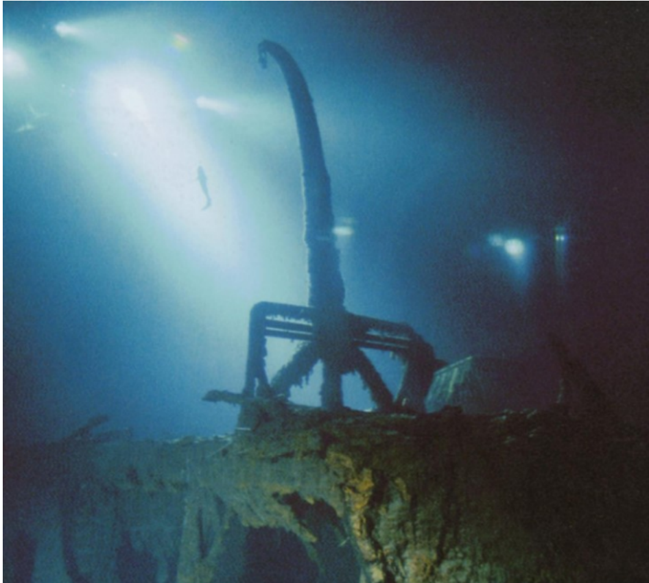
Lifeboat davit 1 is still swung out as if ready to lower another boat.
